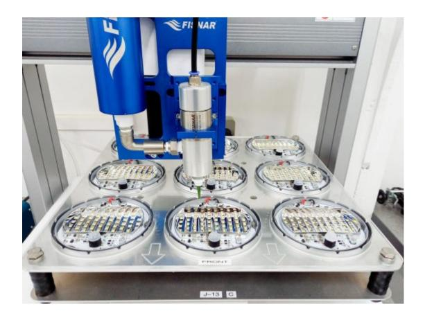
"The robot has sped up our production significantly," said Roderick Dible, Production Manager at Venta Global. "With one skilled operative, our old process would take up to 20 minutes to fully gasket nine lamps. The new set up can do this in less than five."
