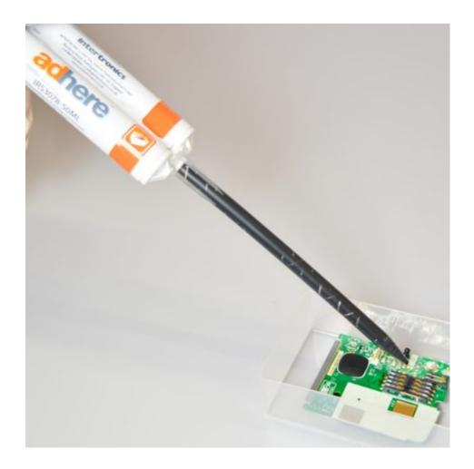
We offer an evaluation kit which contains everything needed to mix and dispense the material - a 50 ml cartridge of epoxy, a dispensing gun and three static mixing nozzles. The material has a 0.90:1 mix ratio by weight, a 1:1 mix ratio by volume and a viscosity of 2,000 mPas. Its working life is six minutes
