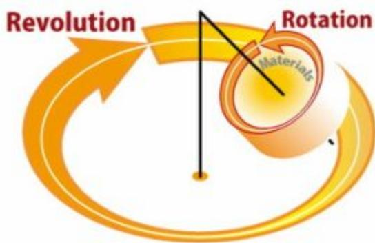
By means of both rotation and revolution of the material in a container, materials are effectively mixed and degassed
