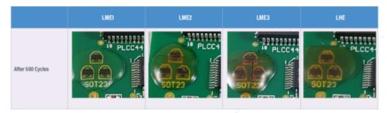
Damp heat and thermal shock tests were carried out
