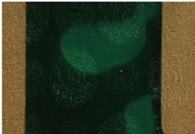
Figure 1 – Grinding away the layers, almost completely through the PCB, uncovers two copper tracks, and in the centre, the remaining solder resist. Under the resist, some voids in the potting compound are apparent.
