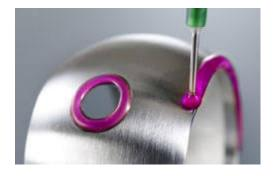
SpeedMask temporary masking compounds are single-part liquids which are readily applied to parts prior to surface treatments. They cure very quickly with UV light, which makes their processing more productive than alternatives like tapes, waxes and solvent-based masks. Their advantages are summarised in this video.
