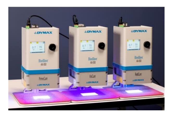
The Dymax AX-550 is available with PrimeCure 385nm, VisiCure 405nm or RediCure 365nm wavelength emitters
