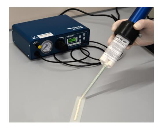
The adhesives are ceramic-filled and thus electrically insulating, two-component products which cure at room temperature. If desired, the cure can be accelerated by heat. The variants differ in their thermal conductivity, temperature resistance and their mechanical properties.
