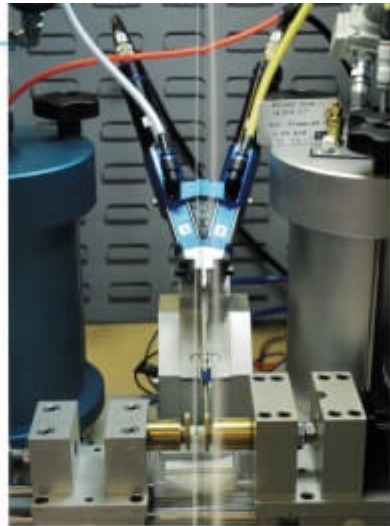
Below: A Parkinson Harwood Technology (PHT) two-part dispensing system, shown in operation.
