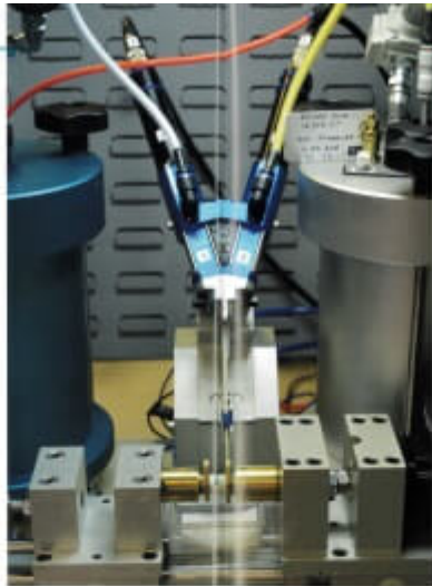
Thomas: A precision use of 3D piezoelectric actuators dispensing system, repeatable and accurate
