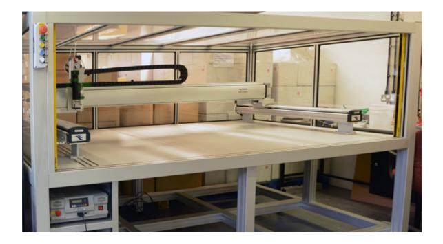
Fisnar F9000 series robots are high power, servo driven, gantry and cantilever style, and are available
