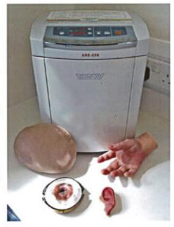
The Thinky solution was excellent for small quantities and also worked particularly well with their system of pre-preparing large batches of colour coded silicone - which was especially arduous and time consuming. The Thinky ARE-250 was found to easily process even highly viscous material, and once programmed ensured a thoroughly mixed, bubble-free compound to the required consistency for every batch without further intervention.
