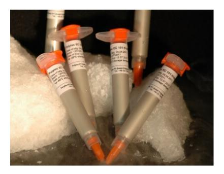
One simple, but nevertheless important, rule must be observed when removing syringes from the freezer: the syringes must only be touched by hand (protected by gloves, of course!) at the flange of the syringe. This is to avoid a local expansion of the syringe wall by uncontrolled heating i.e. by the warmth of your hand – consequently sucking air into the syringe. This may create bubbles inside the syringe and result in voids during dispensing.
