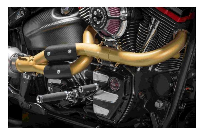
It decided on an <u>Araldite 2031</u> to bond the wide range of materials together, which included metals and thermoset composites, in particular the carbon composite fuel tank to aluminium parts on the front fairings. Where mechanical fasteners, such as rivets added unwanted weight and limited the profile options, the adhesive provided lightweight and greater versatility in design. With its superior
