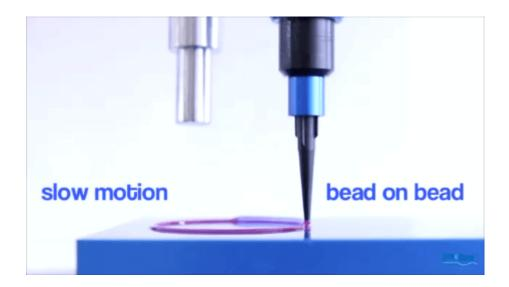
In this illustrative <u>video</u>, a <u>UV curing material from Dymax</u> is applied using a robot fitted with a <u>preeflow eco-PEN precision volumetric dosing unit</u> fitted to a <u>robot</u>. The precisely dosed seal or gasket
