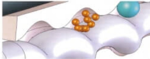
The technology is suited to the pumping, feeding and dosing of fluids which contain microcapsules.
