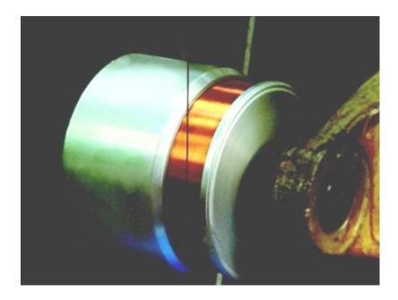
Opti-tec 5054 used for wet winding a coil
