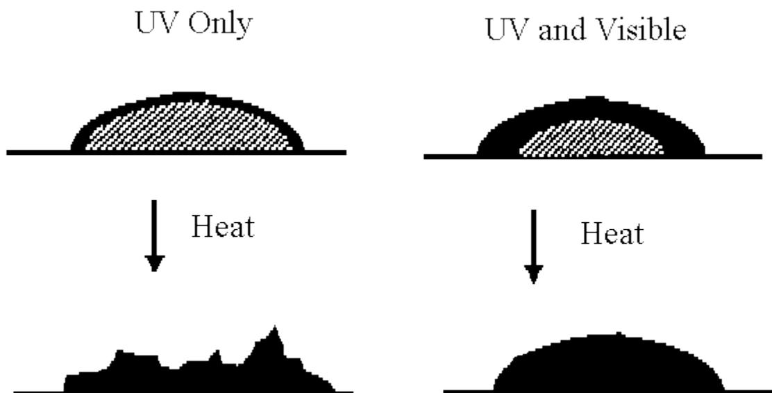
*Figure 5 - Combining UV and visible light for opaque encapsulant cure allows secondary heat cure with no surface eruptions or ripples.*
