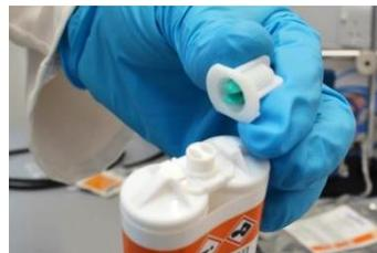
4. Gently squeeze the dispensing gun trigger, and make sure that both of the material components are being pushed out evenly. Wipe off any excess material, and screw on the static mixing nozzle.
