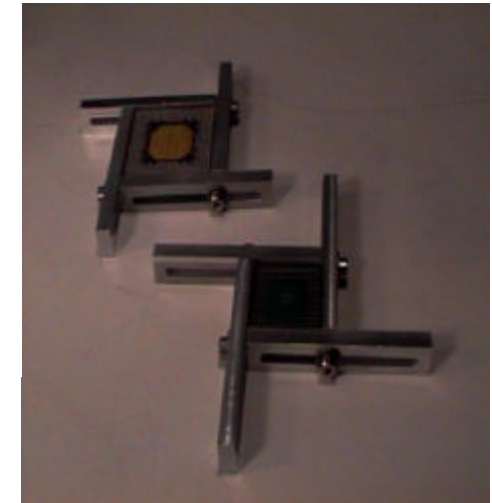
Packages in flexible fixture Size range 5mm to 57mm
