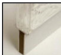
Glass block bonded to plastic with 4-20586
