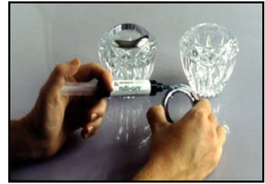
Stainless Steel Trim Bonded to Crystal with DYMAX Light Weld® 619
