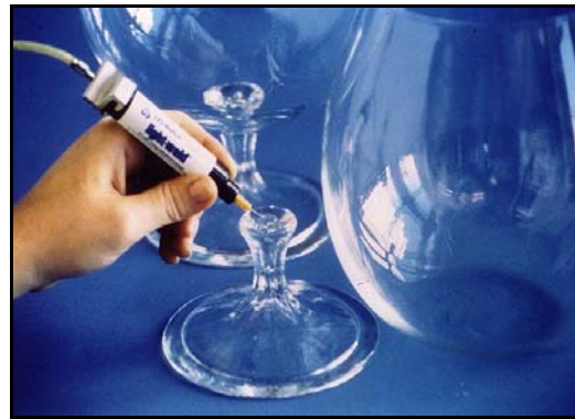
Glass Brandy Snifters Bonded with Crystal Clear, Dishwasher Safe DYMAX Light Weld ® 425
