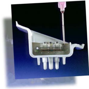
UV/visible potting to 15 mm with acrylate LCMs
