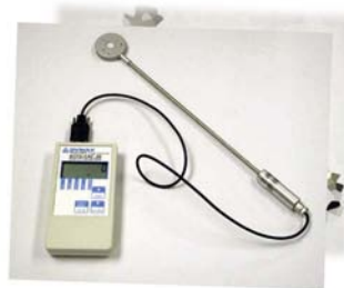
Radiometer equipped to measure the intensity of a flood or spot curing system
