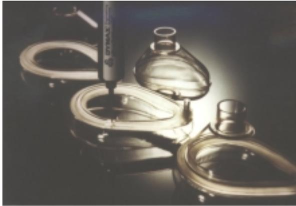
*Figure 6 – Face Mask Bonded with Light Cure Adhesive*
