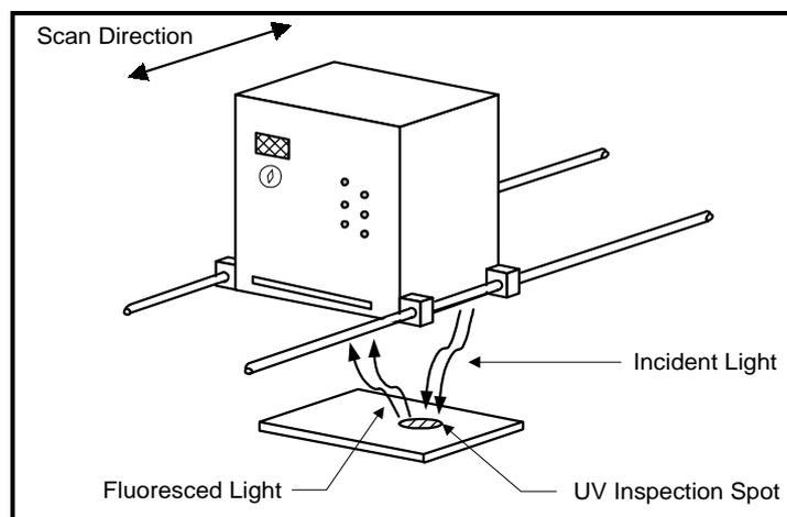
*Figure 4 - On-Line Optical Inspection Scanner*
