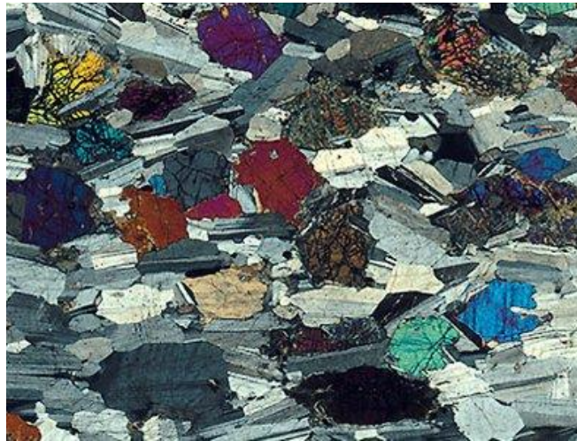
Thin rock section seen through a polarising microscope - various minerals have identifying colours
