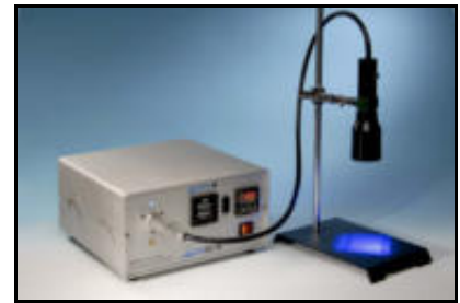
Rod Lenses Shown: BlueWave 200 with 8 mm rod lens (rod lenses require an 8 mm lightguide) 50 mm x 50 mm (2" x 2") Area (~100 mW/cm 2 ) PN 38699 127 mm x 127 mm (5" x 5") Area (~30 mW/cm 2 ) PN 38698
