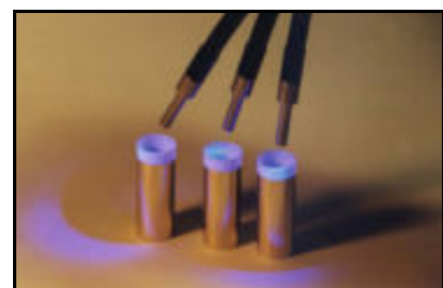
Trifurcated wand curing metal to plastic assembly
