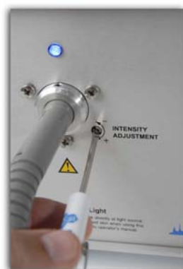
Intensity adjustment, with knob removed, performed with adjustment tool
